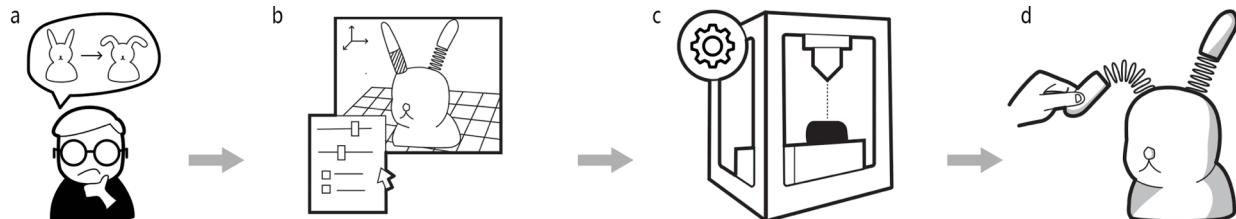
Figure 1: Proposed workflow of making deformable 3D-printed objects – (a) ideating possible deformation behaviors; (b) designing and simulating deformable parts in our CAD tool; (c) fabricating with modified g-code and printer; (d) validating in the real world.
