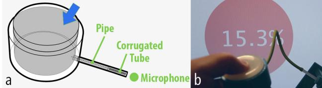
Figure 6. The force sensor: (a) pressing the soft pad generates an air flow; (b) detecting different pressure force.
