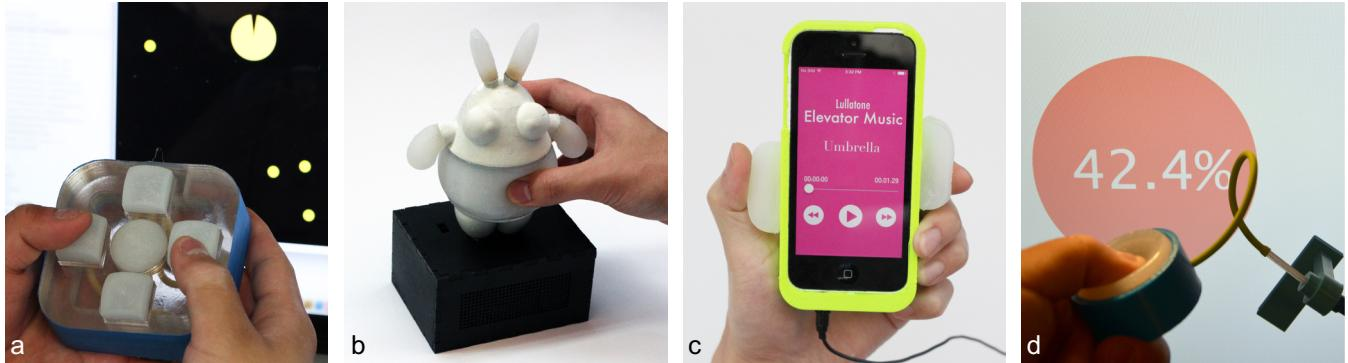
Figure 1. We introduce *Squeezapulse*, a technique for creating interactive fabricated objects using acoustic sensing without external circuitry or power but one single microphone. Above, four example applications show the flexibility and value of our approach: (a) a gamepad controller; (b) a soft and interactive bunny; (c) a squeezable phone case; and (d) a force sensor.
