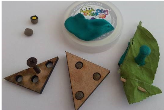
Figure 3 Tangible construction (from top left): a) pen tips with clay inside, b) conductive clay, c) MDF tangible baseplate with screw handle d) underside of the baseplate with pen tips in holes, e) a completed tangible.
