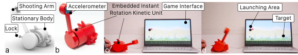
Figure 12: A catapult-like game controller is made to virtually projectile birds in an Angry Birds game: (a) the rendered 3D model of the game controller, (b) the printed game controller with external sensor and circuitry embedded, (c) flying the bird at a small angle, and (d) flying the bird at a bigger angle.
