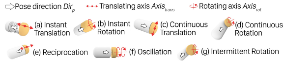
Figure 7: The unit orientation, translation axis, and rotation axis in each kinetic unit. The end-effectors are highlighted in light orange and the stationary parts are marked in grey.
