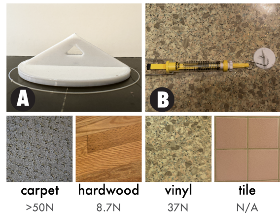
Figure 7: We tested the adhesion strength on four common flooring surfaces—carpet, hardwood, vinyl, and ceramic tile. We printed hooks with a circular base (A) and used a manual force gauge used to measure the force to laterally dislodge the print (B). The prints successfully adhered to all of the surfaces except for the tile.
