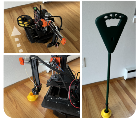
Figure 1: MobiPrint is a custom-built robotic 3D printer that autonomously maps, navigates, and prints 3D objects directly in indoor environments. MobiPrint provides a multi-stage fabrication pipeline: (1) the robotic 3D printer maps an indoor space using LiDAR scanning and obstacle detection; (2) a custom design tool converts the map into an interactive CAD canvas for editing and placing models in the physical world; (3) the MobiPrint robot prints the object directly on the ground at the defined location, as demonstrated in the far-right figure showing a cane holder printed on the floor to prevent it from falling over.
